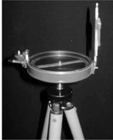
Figure3.1: Prismatic Compass ( Source: www.surveyinginstrumentindia.com )
