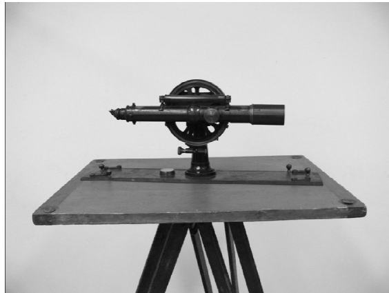
Figure 5.2: Telescopic Alidade on Tripod with Plane Table (Source: www. library2.vicu.utoronto.ca )
